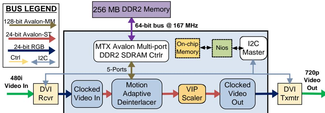
**Figure 5: Block Diagram of HD Deinterlacer/Scaler System**
