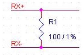
**Figure 4 - LVDS Receive Termination**
