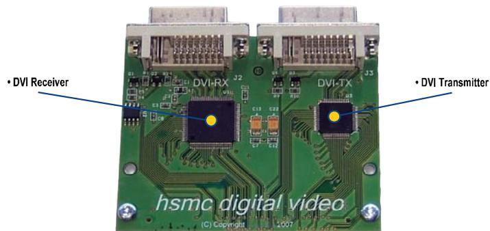
**Figure 3: ViClaro DVI Receiver / Transmitter Board**
