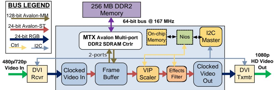
**Figure 7: Block Diagram of HD Dynamic Scaler System**
