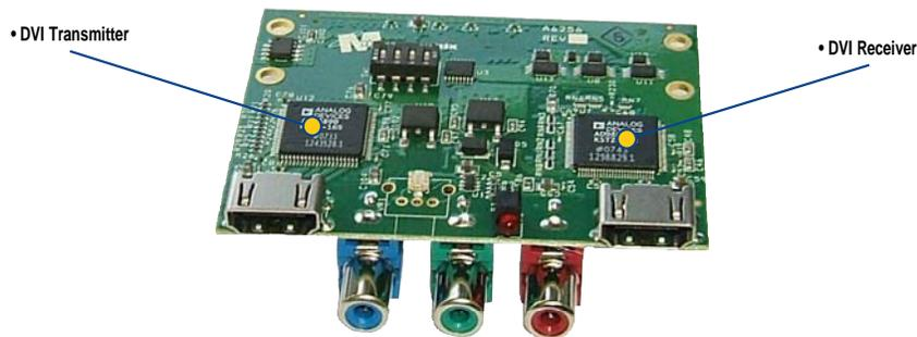
**Figure 2: ViClaro HDMI Receiver / Transmitter Board**
