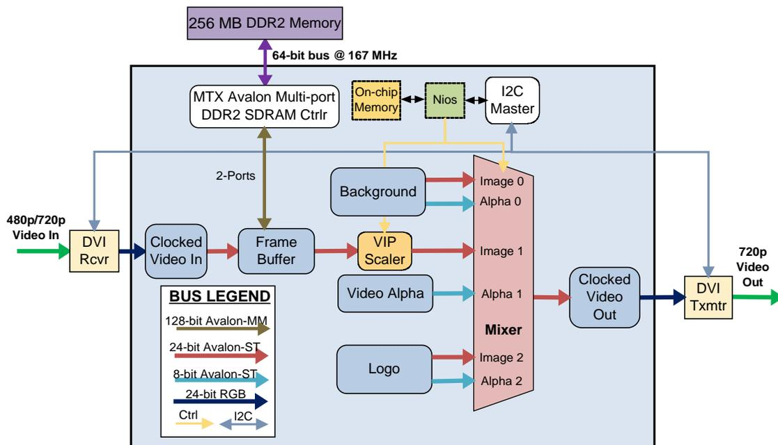
**Figure 8: Block Diagram of HD Mixer System**
