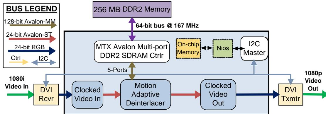
**Figure 6: Block Diagram of HD Deinterlacer System**
