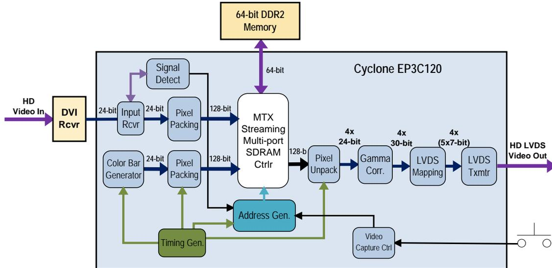
**Figure 9: DVI – LVDS Video Pass-through & Capture**
